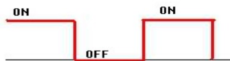
Figure 3. Direct current stimulation. Schematic of the pulse profile, showing constant delivery during “on” period.
