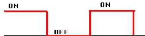
Figure 3. Direct current stimulation. Schematic of the pulse profile, showing constant delivery during “on” period.
