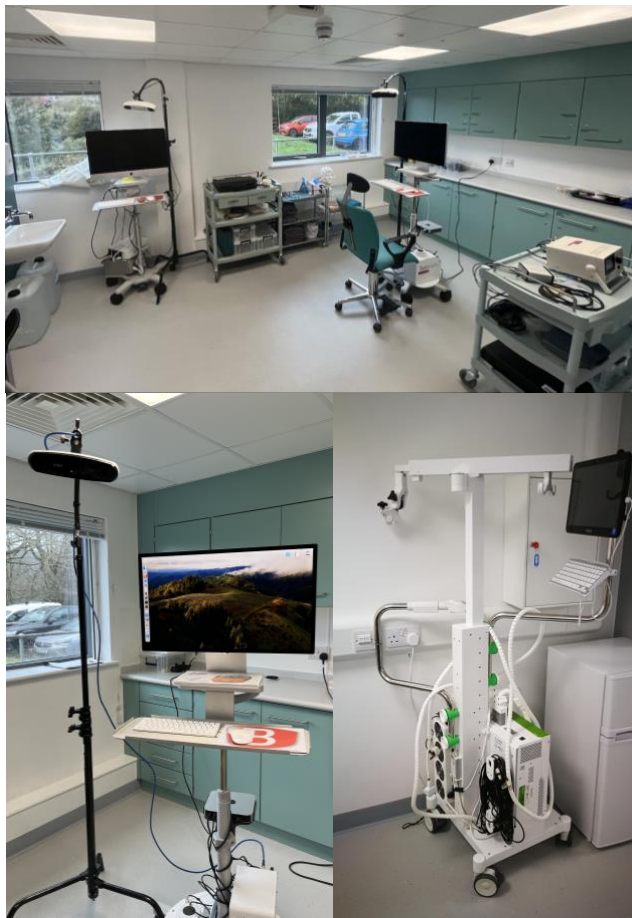
Figure 1. The brain stimulation laboratories at the BRIC. The top image shows the Brain Stimulation Laboratory; The bottom left image shows the Brainsight Neuronavigation system. The bottom right image shows the TMS equipment (DuoMag XT-100, 70mmButterfly Coil (70BF-LQC) with controls and liquid cooling).
