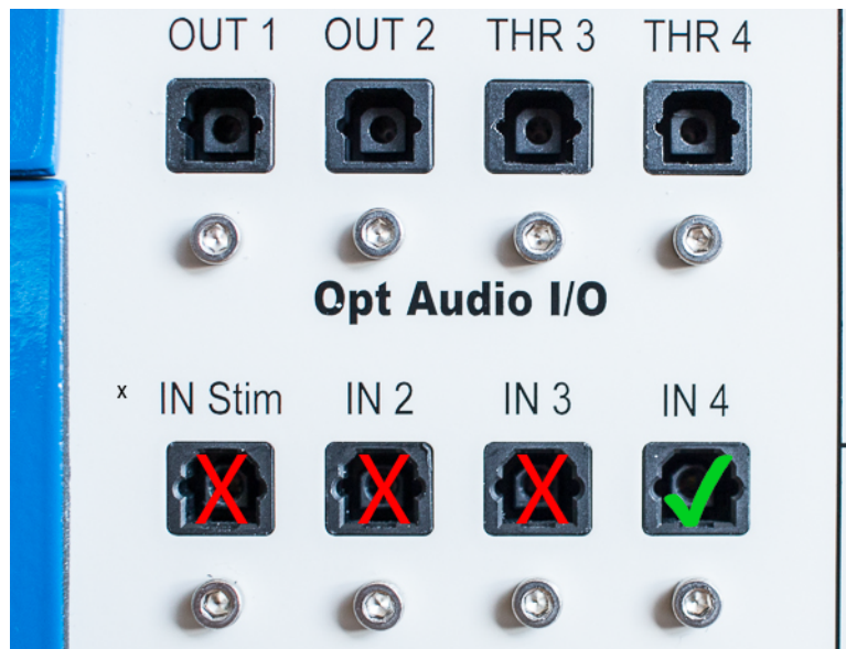
Figure 38 : Installing Optional Feedback Microphone
