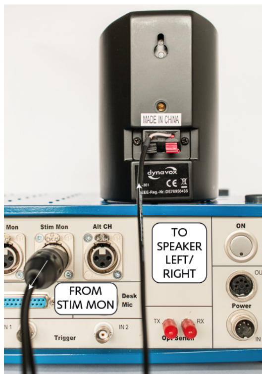
Figure 36 : Rear Speaker installed on the Starter f MKII+ amplifier
