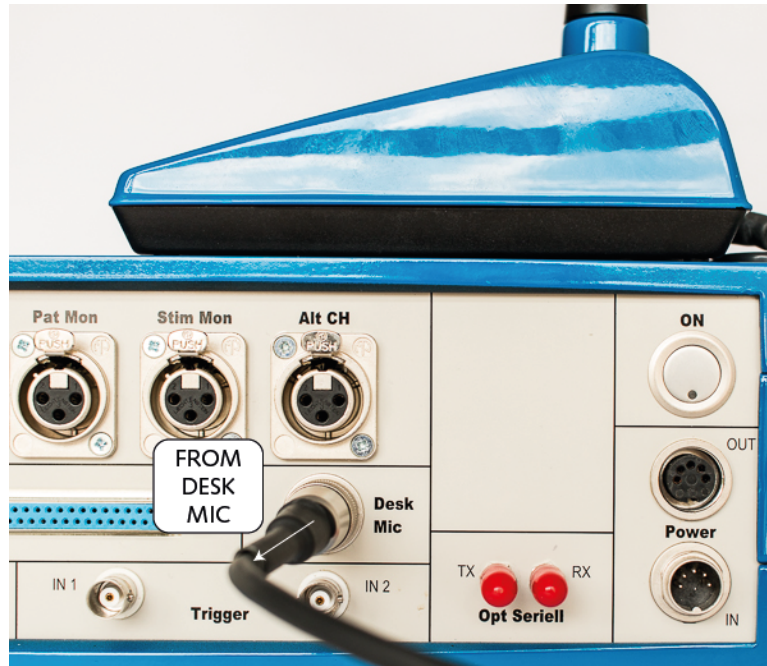
Figure 37: Installing the Technologist microphone
